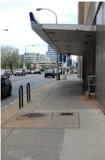
12. Two inverted U racks placed out from under cover are less desirable than the railing, which provides better protection from poor weather.
